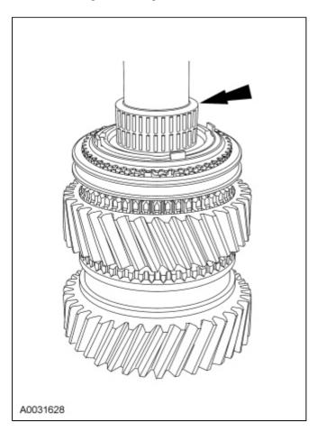
23. **NOTE:** Rotate the gear to align the gear slots with the inner cone tabs.
