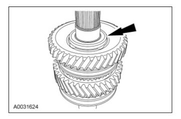
17. **NOTE:** The flatside of 5th gear faces the output shaft end.
