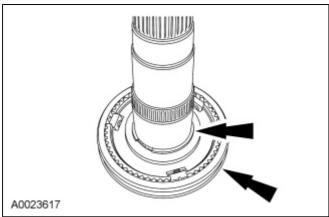
4. **NOTE:** Align the blocking ring tabs with the synchronizer assembly.
