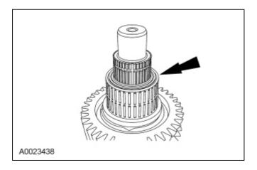
13. **NOTE:** Install the Drive Pinion Bearing Cone Remover behind 2nd gear with the flat side of the tool facing 2nd gear.
