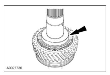
10. Install the reverse gear blocking ring.
