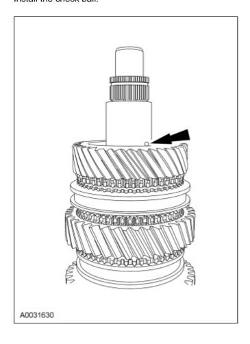
25. Install the thrust washer. Be sure to align the slot in the washer with the check ball.
