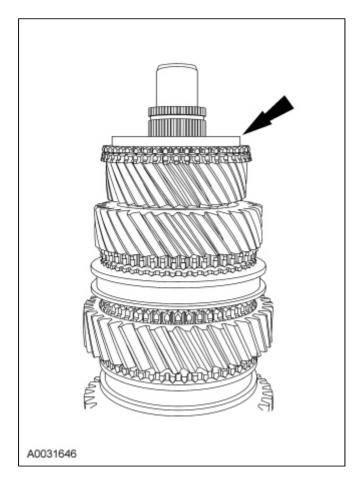
30. **NOTE:** Install the synchronizer body with the raised center facing downward.
