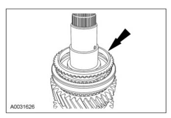
21. Install the 2nd gear synchronizer outer cone and the second gear synchronizer inner cone.
