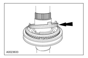
6. Install the inner 1st gear synchronizer cone. Rotate the inner cone until it is seated.
