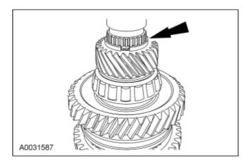
2. NOTICE: Hand-tighten the Drive Pinion Bearing Cone Remover to prevent gear damage.
