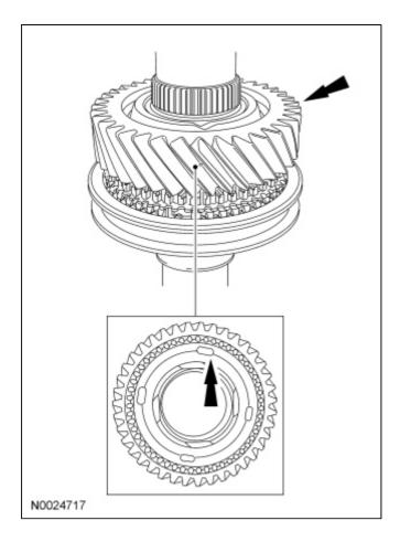
9. Install the reverse synchronizer cone.
