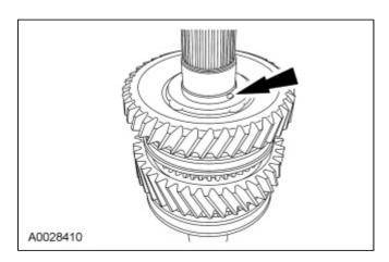
16. Install the thrust washer. Be sure to align the slot in the washer with the check ball.
