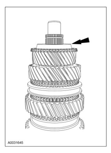
29. Install the 3rd gear synchronizer blocking ring.
