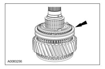
14. **NOTE:** Rotate the gear to align the gear slots with the inner cone tabs.
