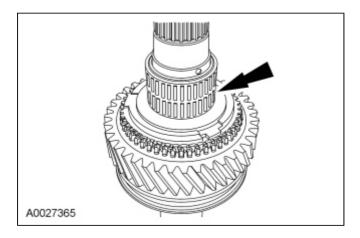
13. Install the reverse gear synchronizer assembly.
