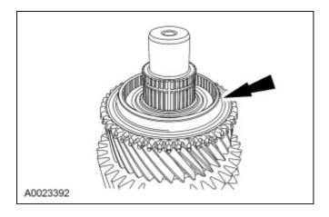
12. **NOTE:** Inspect the needle bearing for wear or damage. Install a new needle bearing as necessary.
