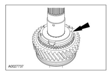
11. Using the Bearing Tube Remover/Installer and Drive Pinion Cone Installer, install the reverse gear bearing spacer.
