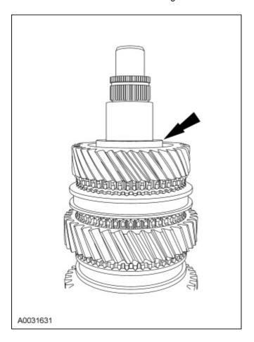
26. Press the bearing spacer onto the output shaft.
