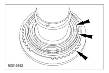
16. Remove and discard the snap ring, then using the Drive Pinion Bearing Cone Remover, press off the 1st/2nd gear synchronizer.
