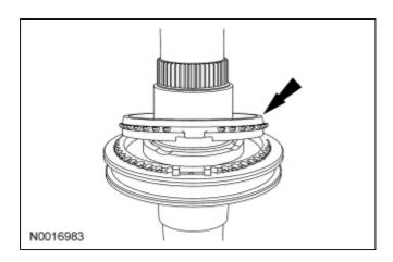
5. Install the outer 1st gear synchronizer cone.
